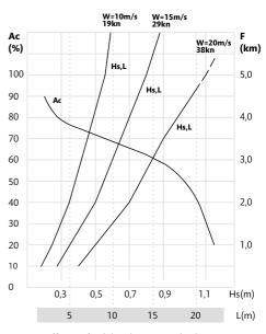
F=Effective fetch lenght. W=Wind velocity.L=Wave length. Hs=Significant wave height.Ac=Wave attenuation capacity.
