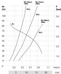
**F**=Effective fetch lenght. **W**=Wind velocity. **L**=Wave length. **Hs**=Significant wave height. **Ac**=Wave attenuation capacity.
